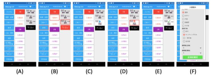
Figure 4-UI of a mobile application for a care record application that using automatic generation function. (A): Initial screen. The estimated care records are shown by gray buttons in the right column, (B): The type of care activity and target patient is entered that was estimated. (C): The state in which the care record was created, (D): doing care activity, (E): Care activity completed, (F): Input the details of records. (F) is already inputted estimated value.
