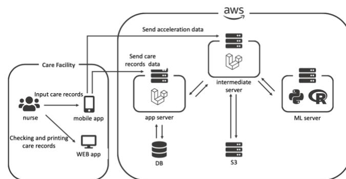
Figure 2-The relationship between mobile applications and servers in care record applications.
